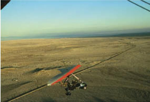
The "trike" is a large, engine-powered hang glider, with a fuselage (including landing gear) suspended from the wing. Instead of launching into the air from the side of a hill, as traditional hang gliders do, the trike is able to self-launch on a level surface by rolling on its wheels and using the power of its rear-mount engine.
