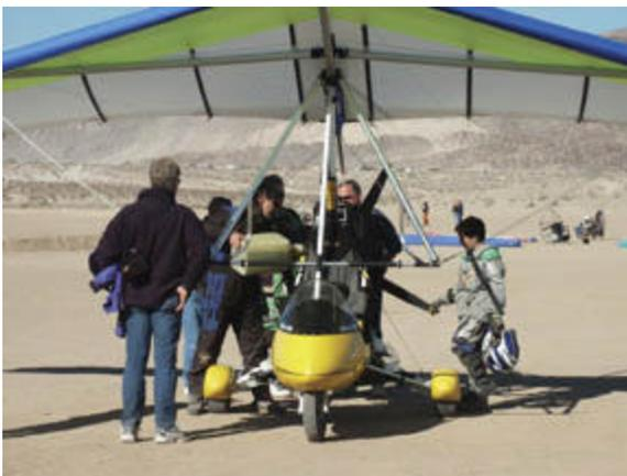
Unlike an airplane, a trike has no tail surface (rudder/elevator) or ailerons. Pitch and roll control are possible by directly changing the angle of the wing with a control bar in front of the pilot. The control inputs are opposite from airplane controls. For example, to flare the trike on landing, the pilot pushes the control bar away from his body, instead of moving the control wheel toward his body.
