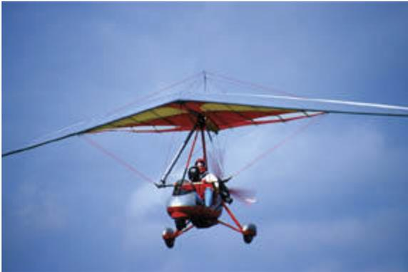
A pilot can also shutdown the engine and soar the trike if the rising thermal is sufficiently strong. However, the lift-to-drag ratio and sink rate of a heavy trike is not as conducive to soaring as a traditional hang glider. To stay aloft, a trike needs rising air of about 450 feet per minute. Lift-to-drag ratio commonly varies from a low of 7:1 to a high of 10:1.
