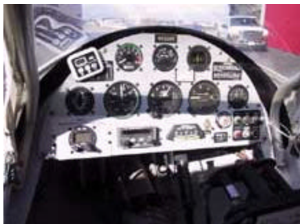
The Becker AN Y201 transceiver is visible in the lower left corner of the front seat instrument panel of the QuickSilver GT-500.
