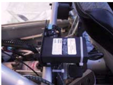
Top view of Sigtronics intercom mounted between front and rear seats. The Becker CU 5209 remote control head is mounted below intercom. The CU 5209 is only 4.2 inches long.
