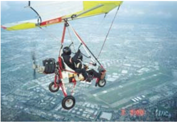
Jon Thornburgh flies a glider-trike over Torrance Airport. Note the control column extension bars used for instruction in the back seat.
